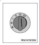
(1) It is possible to control the fan speed as four steps.
