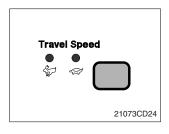
① This switch is to control the travel speed which is changed to high speed(Rabbit mark) by pressing the switch and low speed(Turtle mark) by pressing it again.
