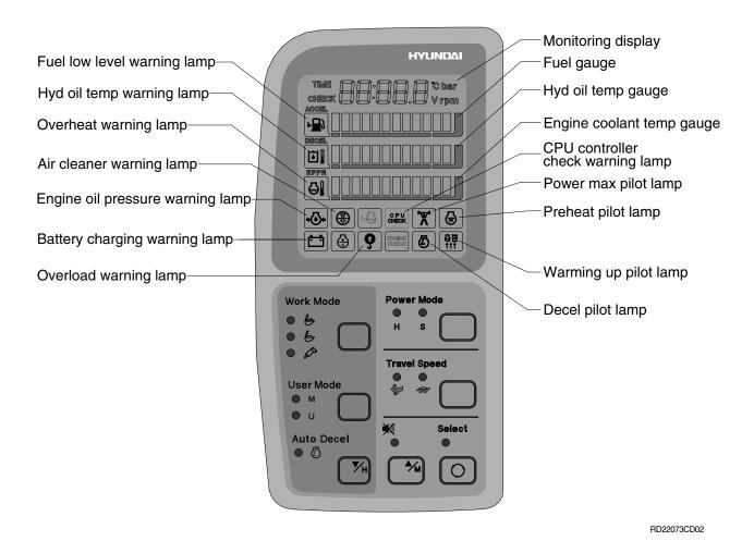
\* The warming lamp lights ON and the buzzer sounds when the machine has a problem.
