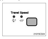
① This switch is to control the travel speed which is changed to high speed(Rabbit mark) by pressing the switch and low speed(Turtle mark) by pressing it again.
