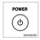
① Press ① to switch ON the set. Press ① for more than 2seconds to switch OFF the set.
